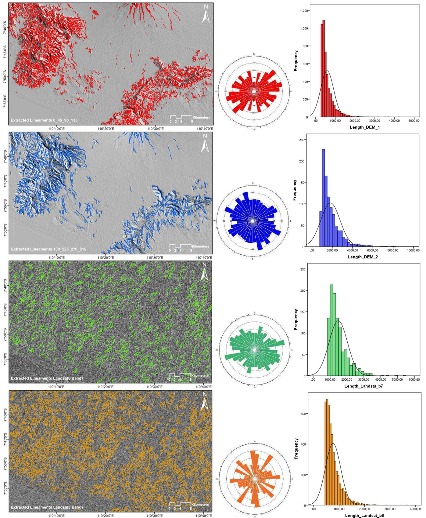
Fig. 4. Imagery from DEM and Landsat 8 imagery analyze different light azimuth of  $0^{\circ}$ - $45^{\circ}$ - $90^{\circ}$ - $135^{\circ}$  (DEM 1);  $180^{\circ}$ - $225^{\circ}$ - $270^{\circ}$ - $315^{\circ}$  (DEM2); band 7 and band 8 of Landsat 8. Each lineaments trend differently has its direction with length frequency distribution shows each histogram.
