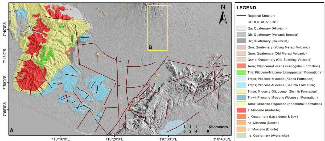
Fig. 2. Geological map with a regional structure of the southern part of Merapi in Yogyakarta. Geological Research and Development Center provided Geological information [22]. (B) Small scale for Hill-shaded images with lighting from various azimuth angle.
