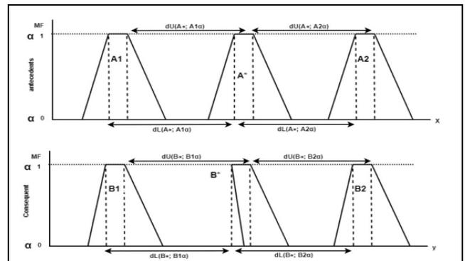
Fig.2: Fuzzy Interpolative Reasoning with an Invalid Conclusion for The KH FRI
