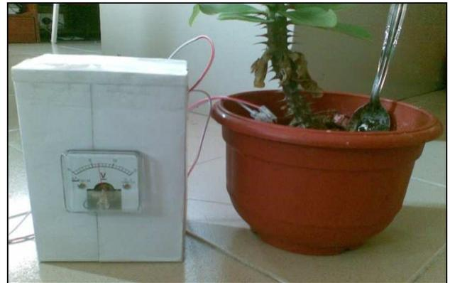
Fig. 11 Water detector unit
