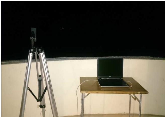
Fig. 3 Setting of the SQM device for ground measurements of sky brightness in the study area
