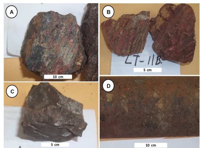
Fig. 2 Chip samples of ultramafic rocks from Latowu showing brown to reddish-brown in color, indicating elevated concentration in iron oxides.
