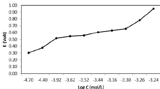
Fig. 12 Graph of MIP potential of endosulfan to the target of logarithm concentration on the aluminum-carbon electrodes on at 20<sup>th</sup> day
