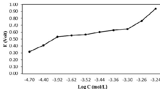
Fig. 11 Graph between MIP endosulfan potential to the target logarithm concentration on the aluminum-carbon sensor on the 1<sup>st</sup> day
