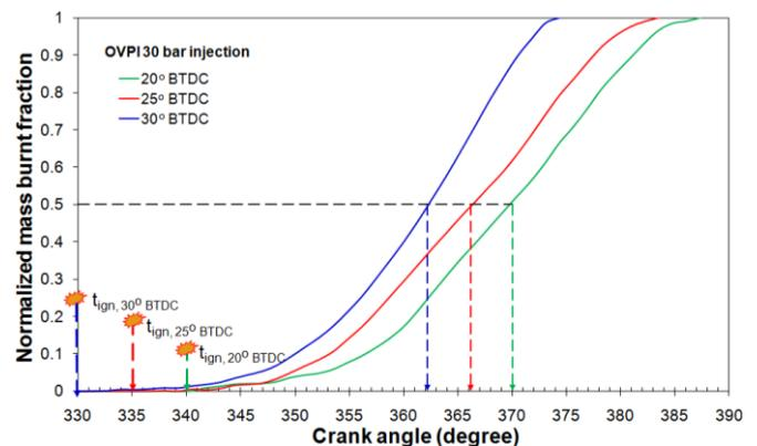
Fig. 13 Mass burnt fraction for OVPI at various ignition timings
