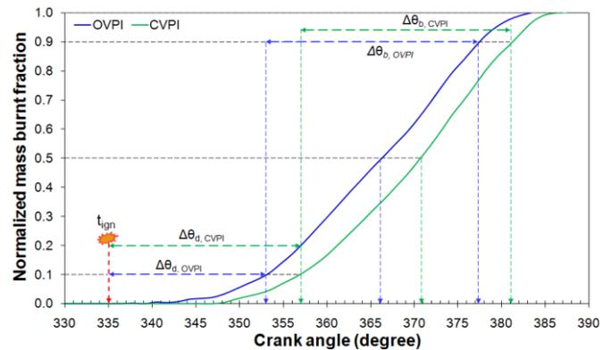
Fig. 12 Mass burnt fraction for OVPI and CVPI
