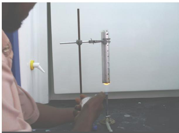
Fig. 1 Flammability test using the vertical burning column
