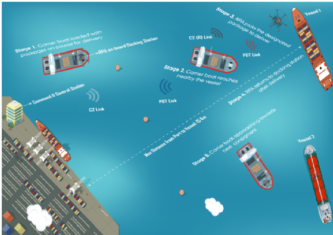
Fig. 5 The proposed system architecture for the automation of the end-to-end delivery process [48]
