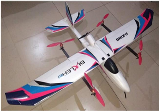
Fig. 1 Separate-lift-and-thrust hybrid drone
