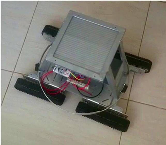
Fig. 2 ARMOS TurtleBot 1 robot. This robot is 45 cm wide and 61 cm long. Around its vertical axis, it has nine infrared distance sensors distributed along a circular aluminum bar, with 40 degrees of separation one from the other. These sensors have a range of 0.2 to 0.8 m
