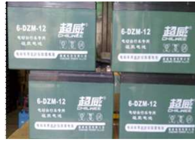
Fig. 6. Accumulators used as power source for the motorcycle
