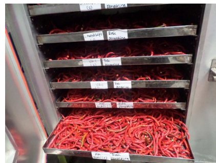
Fig. 3 Cabinet drying at 50-60 °C
