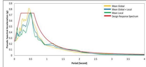
Fig. 11 Recommended Design Response Spectrum for Soil Type C
