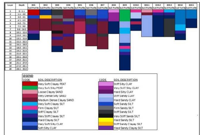
Fig. 4 The Soil Profile for 15 Boreholes
