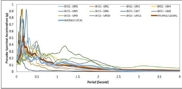
Fig. 6 Response Spectra at Surface for Soil Type A
