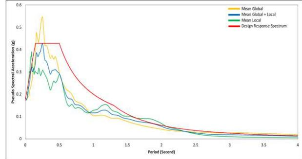
Fig. 10 Recommended Design Response Spectrum for Soil Type B
