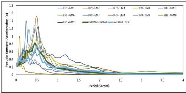
Fig. 8 Response Spectra at Surface for Soil Type C
