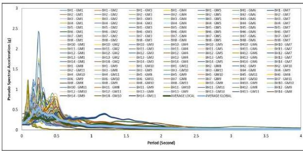
Fig. 7 Response Spectra at Surface for Soil Type B
