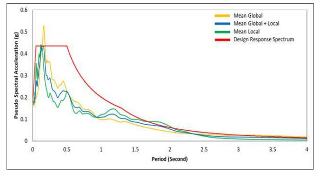
Fig. 9 Recommended Design Response Spectrum for Soil Type A
