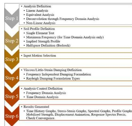
Fig. 5 Analysis Stages in DEEPSOIL Software [36]
