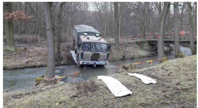
Fig. 3 Passes of the vehicle with plastic mats – both directions [25]
