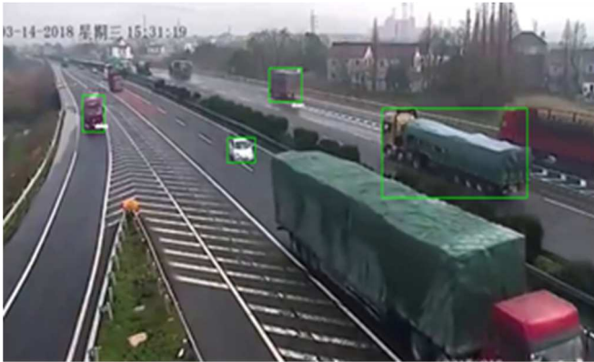
Fig. 4 Wrong direction detection in low resolution video
