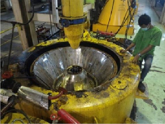
Fig. 1 Conical continuous centrifuges
