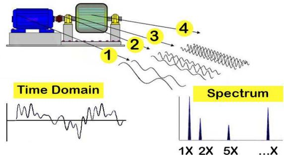
Fig. 2 Vibration frequency extraction
