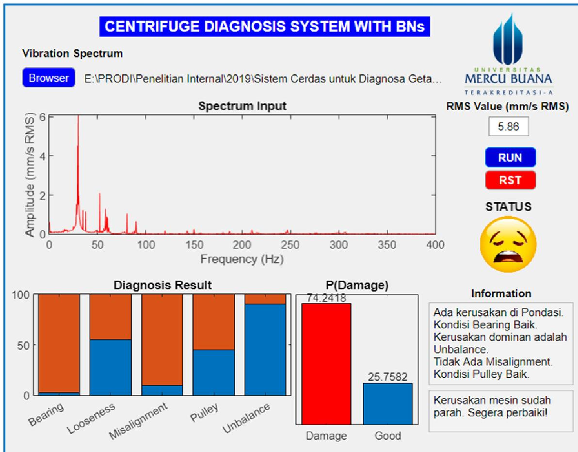
Fig. 8 System testing
