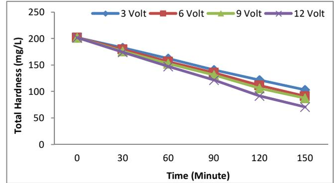
Fig. 17 The Effect of Electrocoagulation Process on Total hardness reduction
