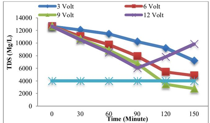
Fig. 5 The Effect of Electrocoagulation Process on TDS reduction
