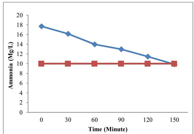
Fig. 9 Effect of the adsorption process on Ammonia reduction
