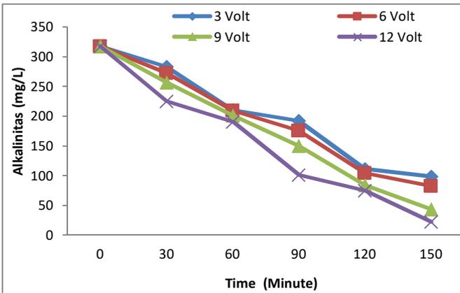
Fig. 16 Effect of Combination Process between Electrocoagulation and Adsorption on Alkalinity reduction
