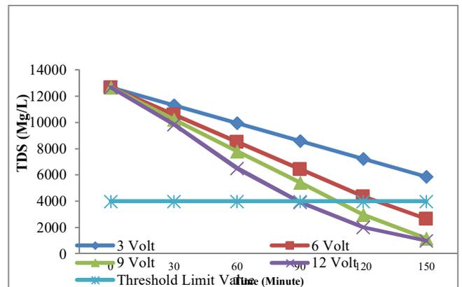
Fig. 7 Effect of Combination Process between Electrocoagulation and Adsorption on TDS reduction
