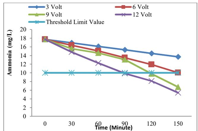
Fig. 10 Effect of Combination Process between Electrocoagulation and Adsorption on Ammonia reduction
