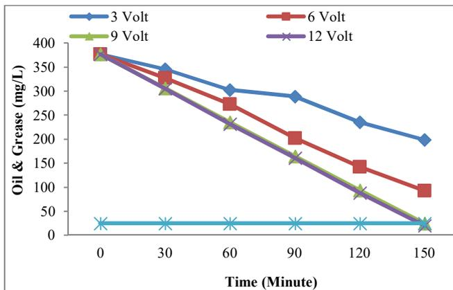
Fig. 11 The Effect of Electrocoagulation Process on oil & grease reduction
