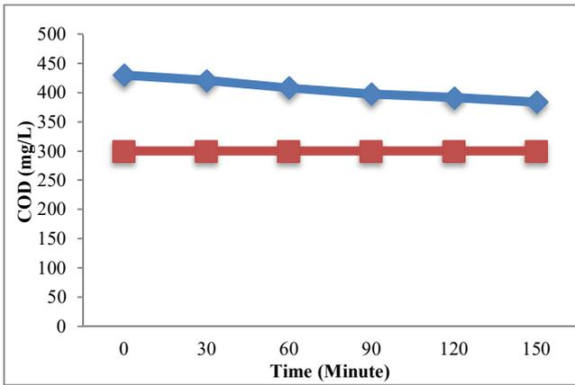
Fig. 3 Effect of the adsorption process on COD reduction
