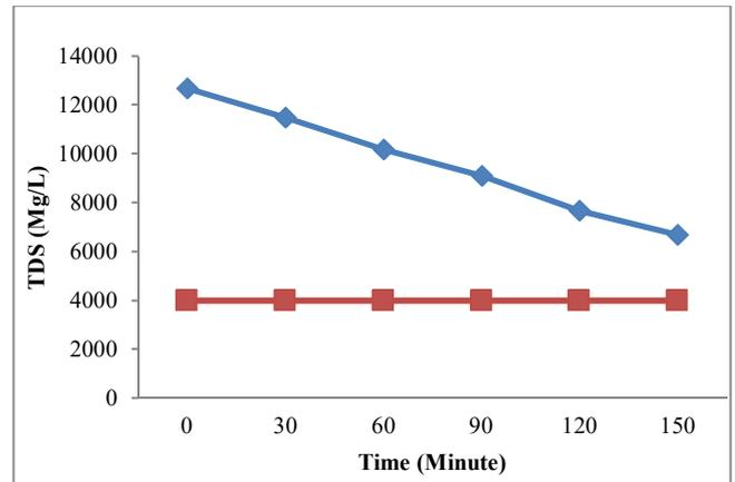
Fig. 6 Effect of the adsorption process on TDS reduction
