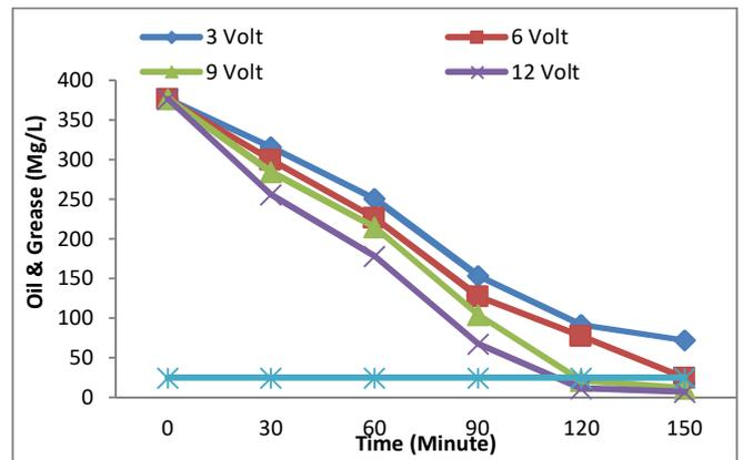
Fig. 13 Effect of Combination Process between Electrocoagulation and Adsorption on oil & grease reduction
