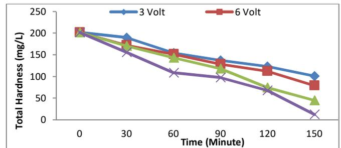
Fig. 19 Effect of Combination Process between Electrocoagulation and Adsorption on Total hardness reduction
