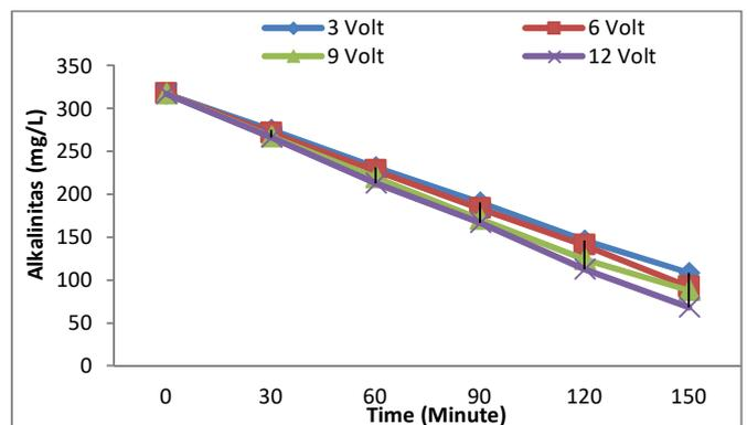
Fig. 14 The Effect of Electrocoagulation Process on Alkalinity reduction
