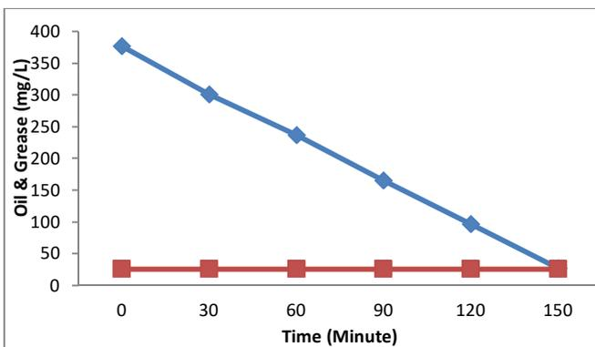
Fig. 12 Effect of the adsorption process on oil & grease reduction
