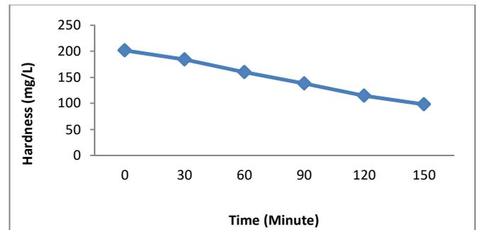
Fig. 18 Effect of the adsorption process on Total hardness reduction
