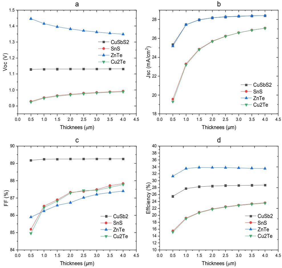
Fig. 3 (a) VOC vs. absorber layer thickness; (b) JSC vs. absorber layer thickness; (c) Fill factor vs. absorber layer thickness; (d) Efficiency vs. absorber layer thickness.
