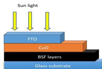
Fig. 1 Schematic diagram of CuO solar cell.
