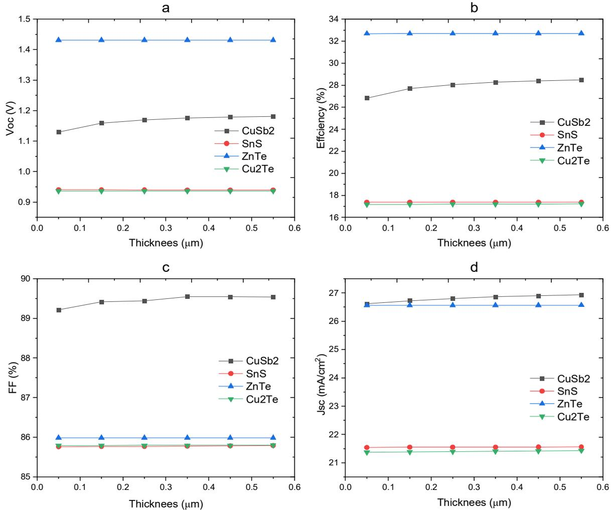
Fig. 2 (a) VOC vs. BSF layer thickness; (b) JSC vs. BSF layer thickness; (c) Fill factor vs. BSF layer thickness; (d) Efficiency vs. BSF layer thickness
