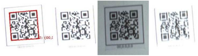
Fig. 12 QR code images respectively at exposure value H 2.76, 3.18, 1.05, and 2.76 lux·s, motion blur MB 3.8, 3.8, 3.8, and 14.5 pixels, and recall 63.26%, 54.29%, 31.25%, and 0.61%
