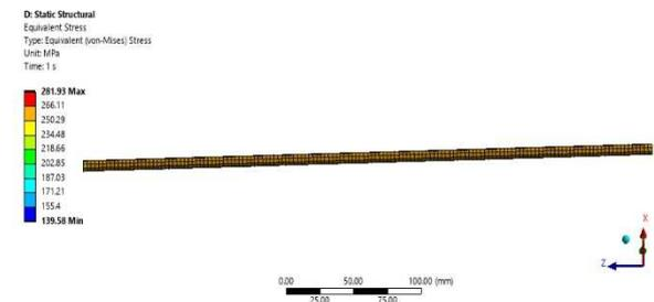
Fig. 11 Von Mises Stress Distribution of 304 Stainless Steel
