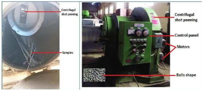
Fig. 2 Shot peening test rig
