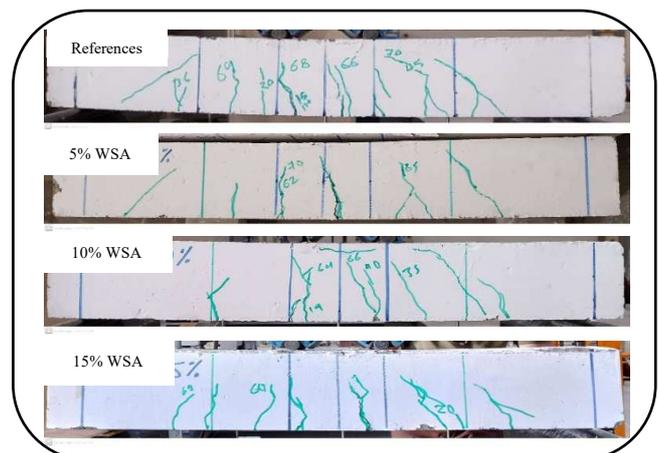
Fig. 14 Crack pattern and shape of failure for beams in Group 1
