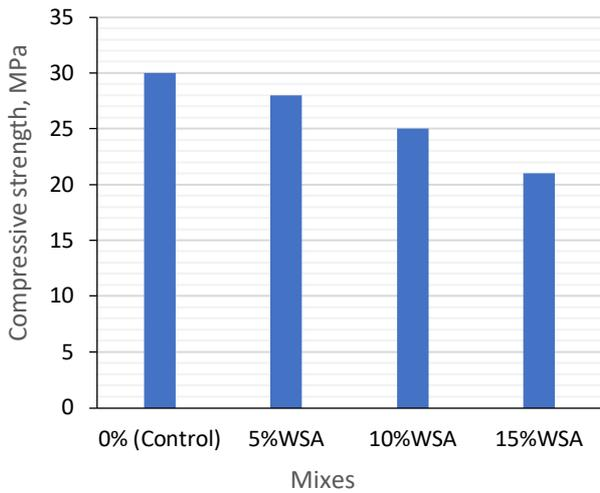
Fig. 5 Compressive strength vs. WSA%
