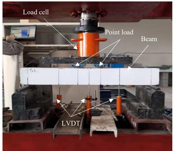
Fig. 3 Procedure for preparing of beams for testing
