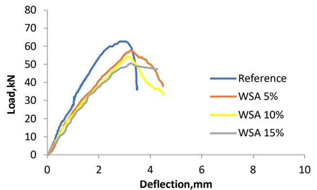
Fig. 7 Load-deflection vs. WSA% in shear
