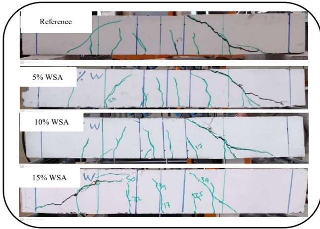
Fig. 15 Crack pattern and shape of failure for beams in Group 2
