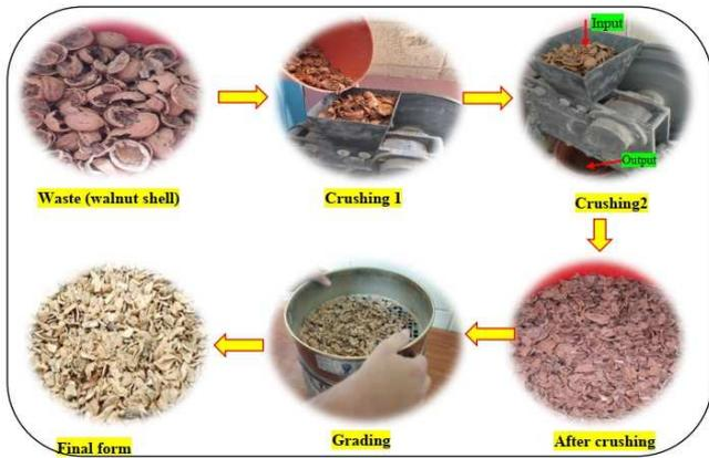
Fig. 1 Procedure for WSA preparing
