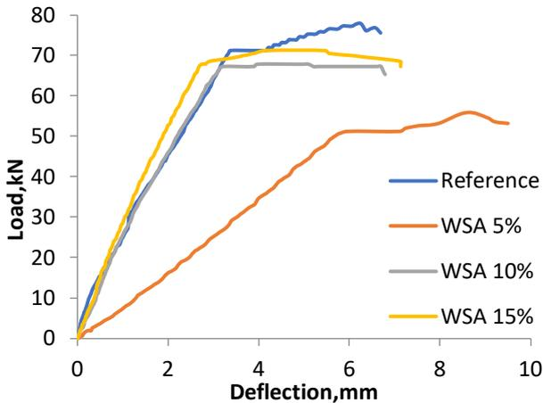
Fig. 6 Load - deflection vs. WSA% in flexural
