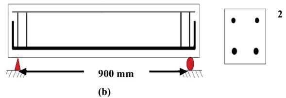
Fig. 4 Reinforced details (a) for flexural failure (b) for shear failure
