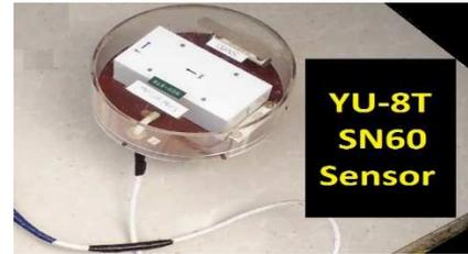
Fig. 8 The Installation of YU-8T Magnetometer Sensor
