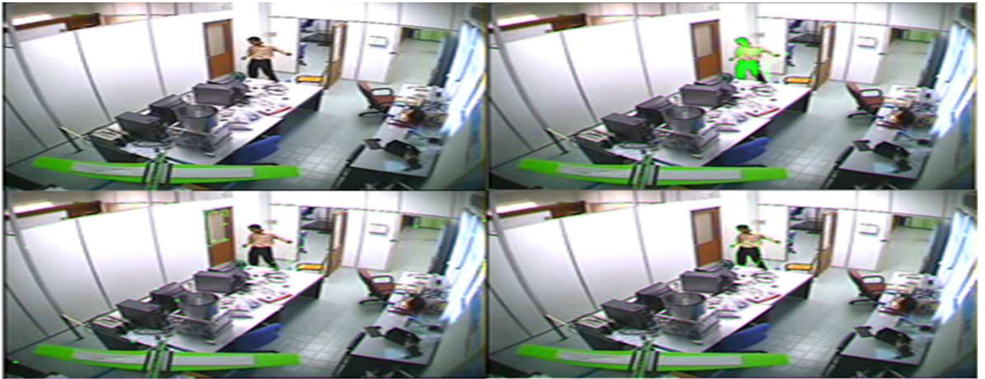
Fig. 5 Motion detector comparison: (Clockwise) original image, simple background subtraction (two frame differences), proposed technique and low precision background subtraction
