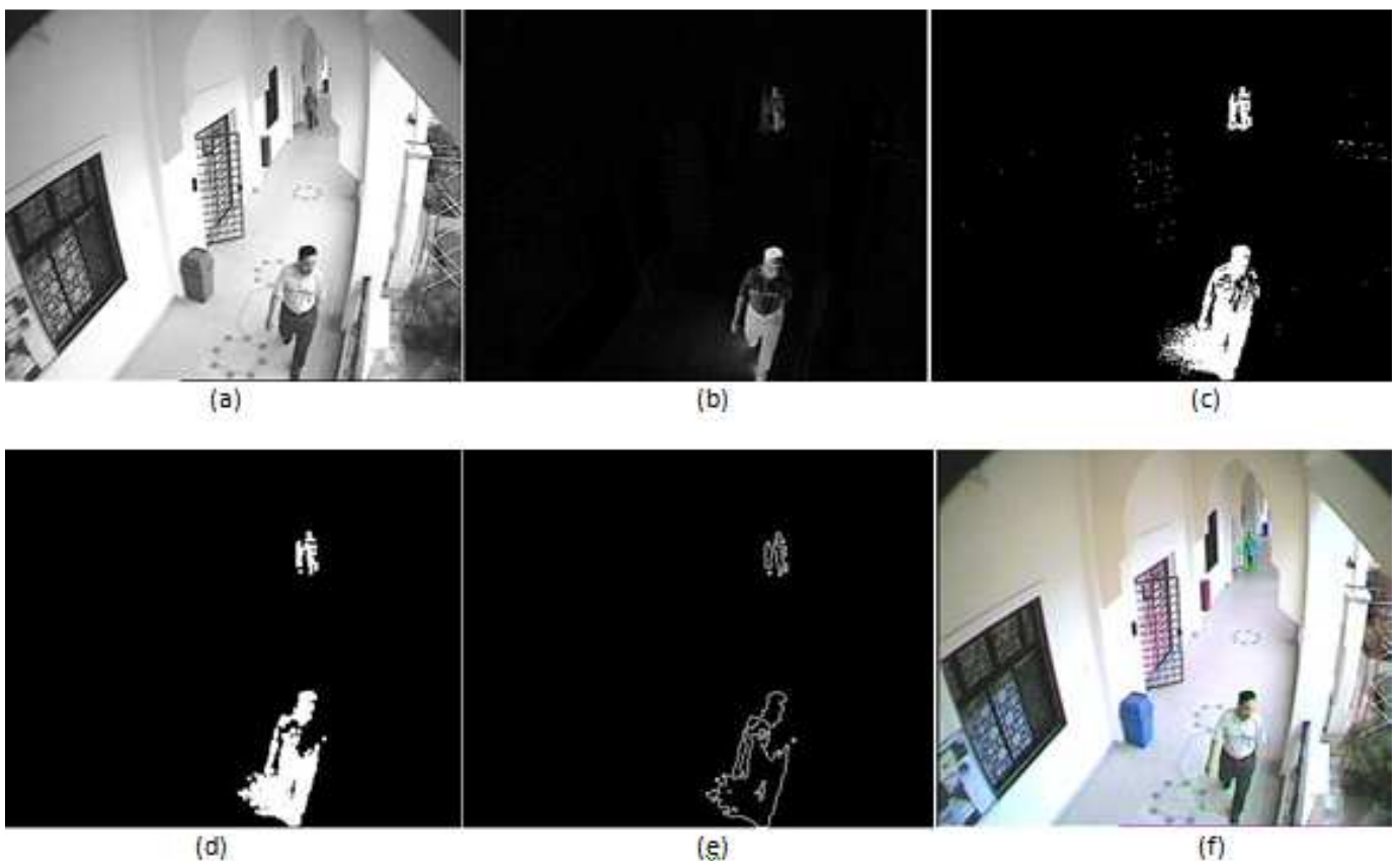
Fig. 2 Image processing in proposed technique: (a) Grayscale (b) Background subtraction (c) Thresholding (d) Opening filter (e) Edge filter (f) Final image with motion region boundaries
