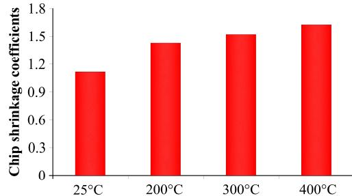
Fig.6. Chip shrinkage coefficients at different heating experiments
