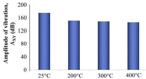
Fig.10 Amplitude of vibration when machining at different temperature conditions
