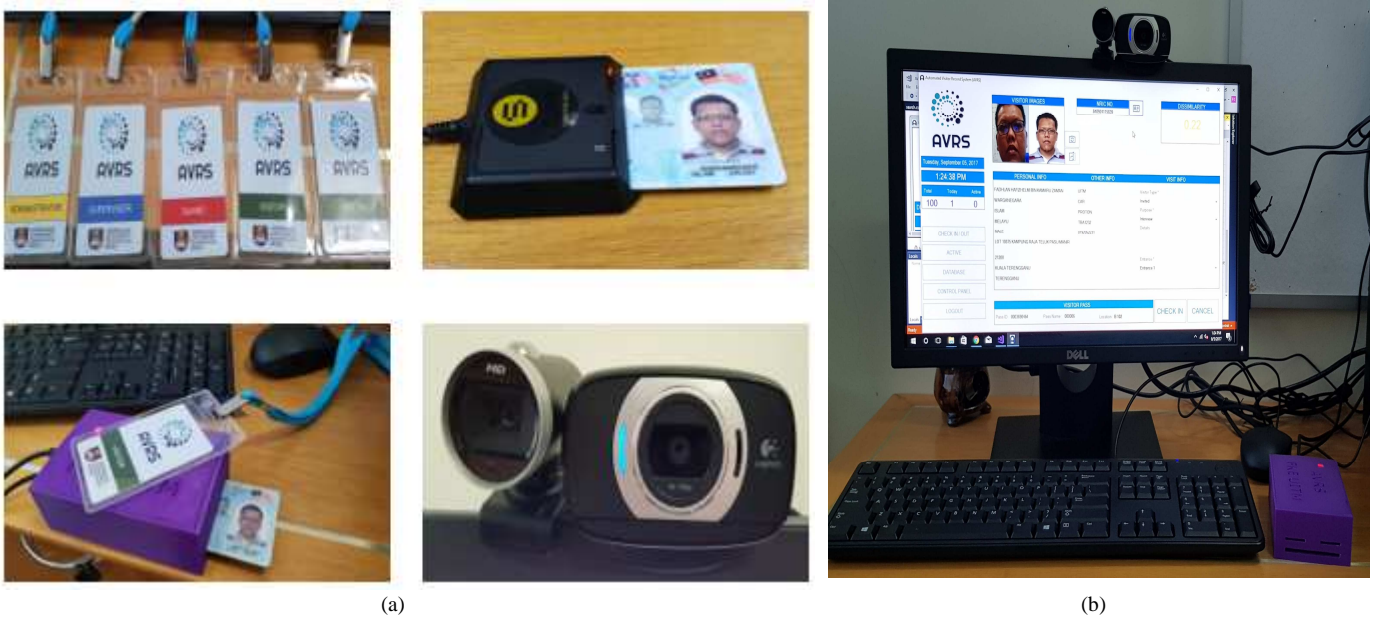
Fig. 2 The hardware used to build the system. (a) (following clock cycle) from top left is RFID cards, Smart card reader with an NRIC attached, 125KHz RFID reader and webcams. (b) The complete setup of the proposed system with its hardware and a PC
