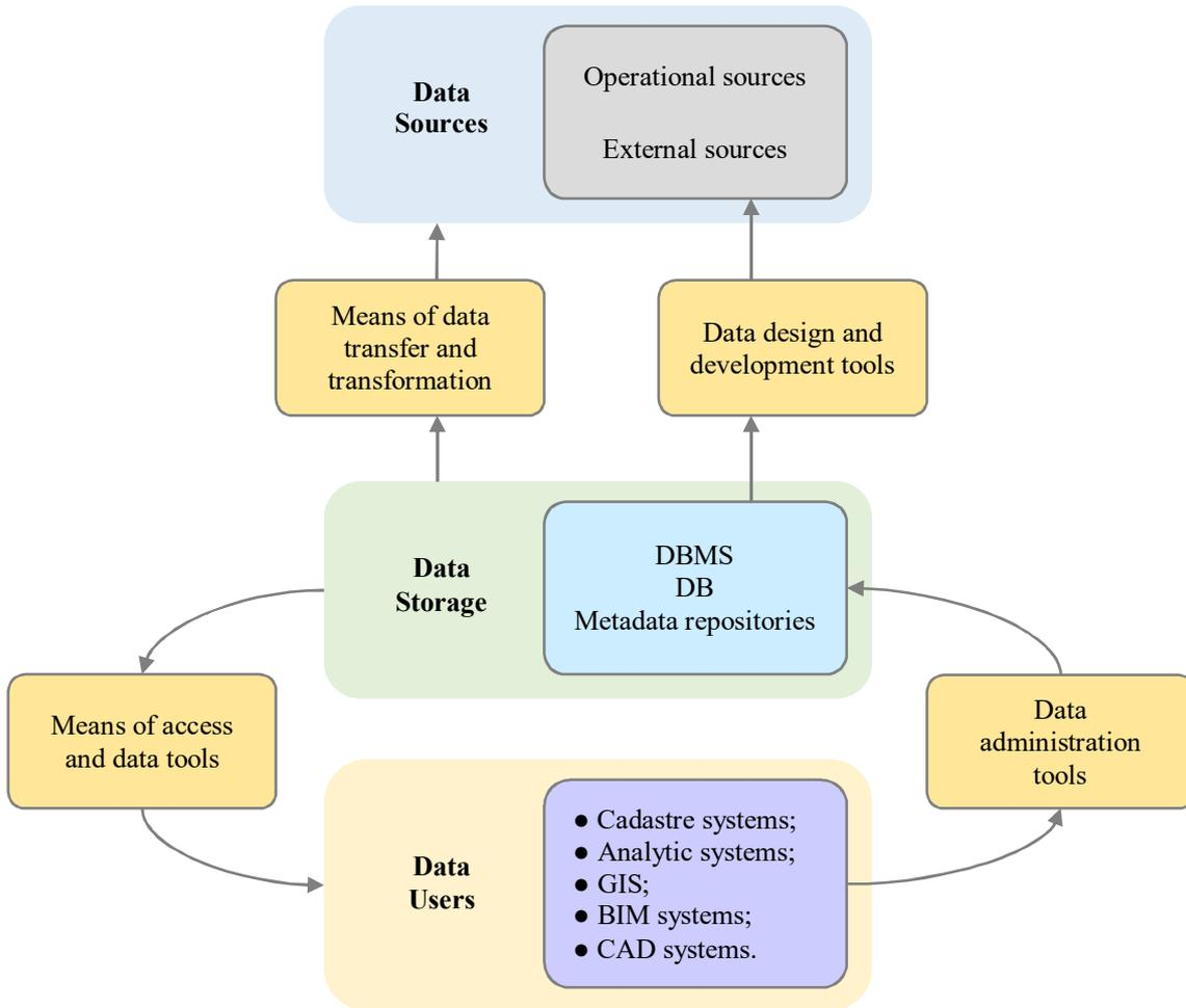
Fig. 3 BIM-model of spatial and attribute data integration
