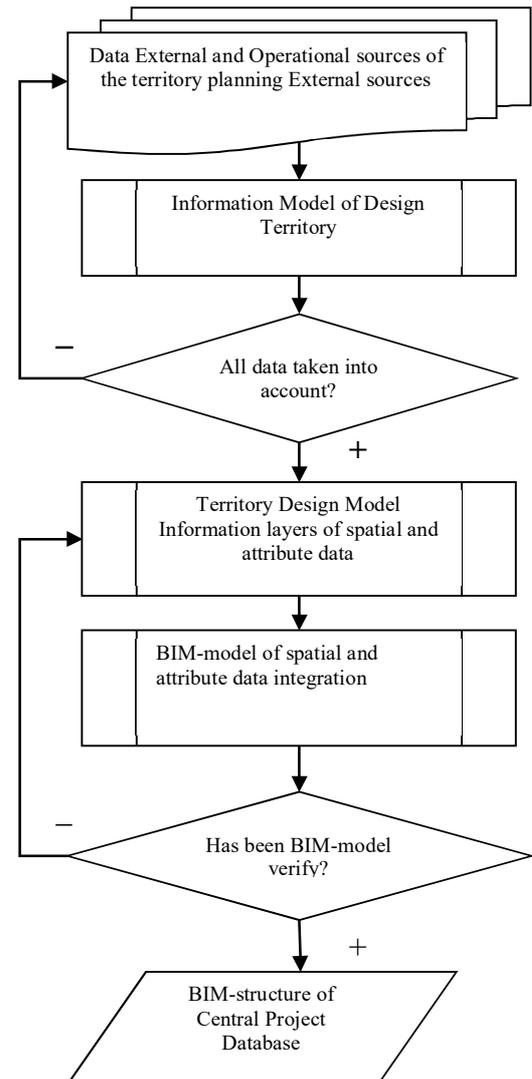
Fig. 1 Block diagram of the creation BIM-structure of Central Project Database
