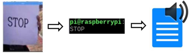
Fig. 11 The block diagram for text-to-speech process. (a) a test image, (b) captured letters on notepad, and (c) speech out with text.txt file
