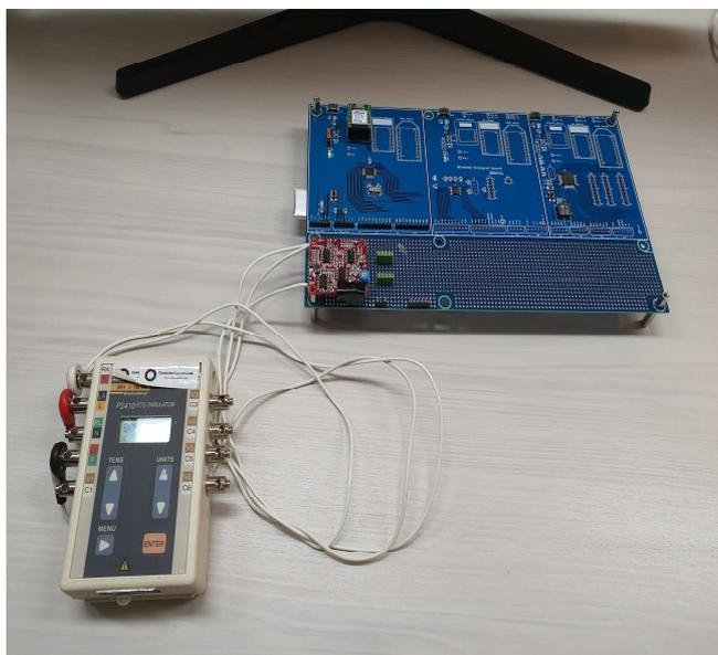
Fig. 1 Collect ecg data using arrhythmia generator and ecg sensor
