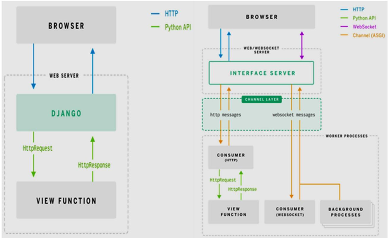
Fig. 20 Existing communication methods (left) and methods using websocket (right)
