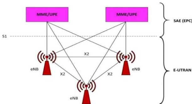
Fig. 1 LTE network architecture: E-UTRAN access network and SAE core network
