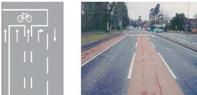
Fig. 4 Bike boxes with a central cycle lane [19]
