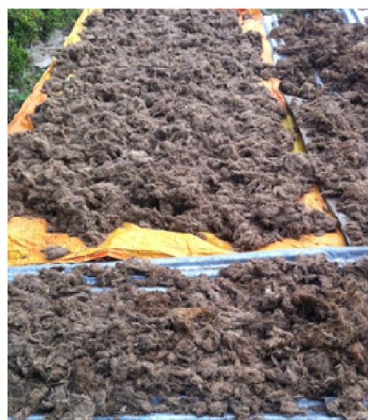
Fig. 3 EFB of dried in open sun drying
