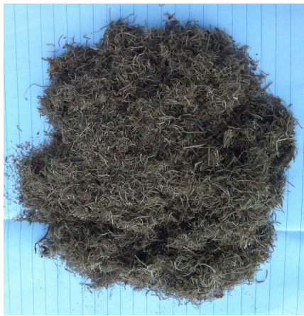
Fig. 4 Empty Fruit Bunch powder and fiber
