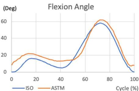
Fig. 1 Knee joint extension flexion according to ISO142431 and ASTM F3141-17
