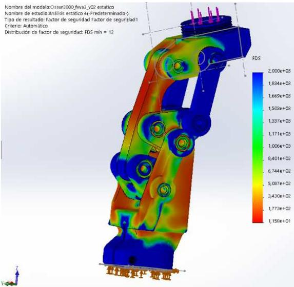
Fig. 15 Finite element simulation of the Ossur 2000 knee joint.
