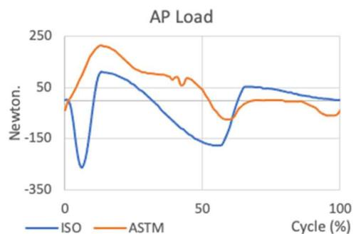
Fig. 6 Anterior-posterior loading under ISO142431 and ASTM F3141-17
