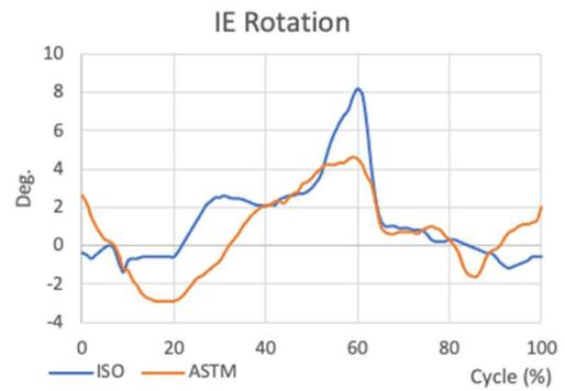
Fig. 3 Internal - external angle according to ISO142431 and ASTM F3141-17
