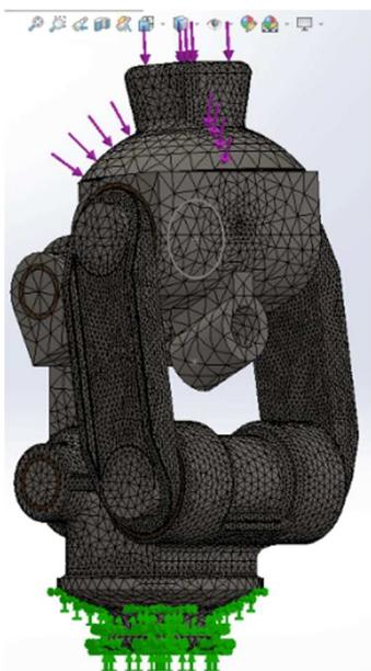
Fig. 17 Streifeneder 3A20 knee joint digitization
