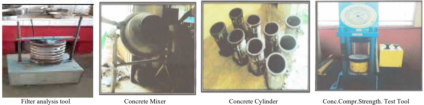
Fig. 2 Equipment for making cylindrical concrete samples
