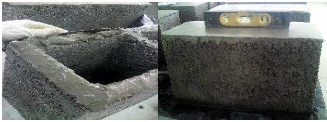
Fig. 4 Placing mortar on the upper face of the block (left); leveling the mortar placed on the lower part of the block (right).
