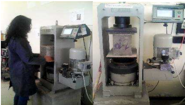
Fig. 6 Placing hollow concrete block in compression machine.
