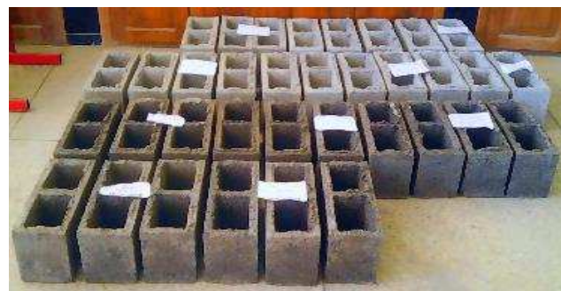
Fig. 3 Curing and storage process of hollow concrete blocks.
