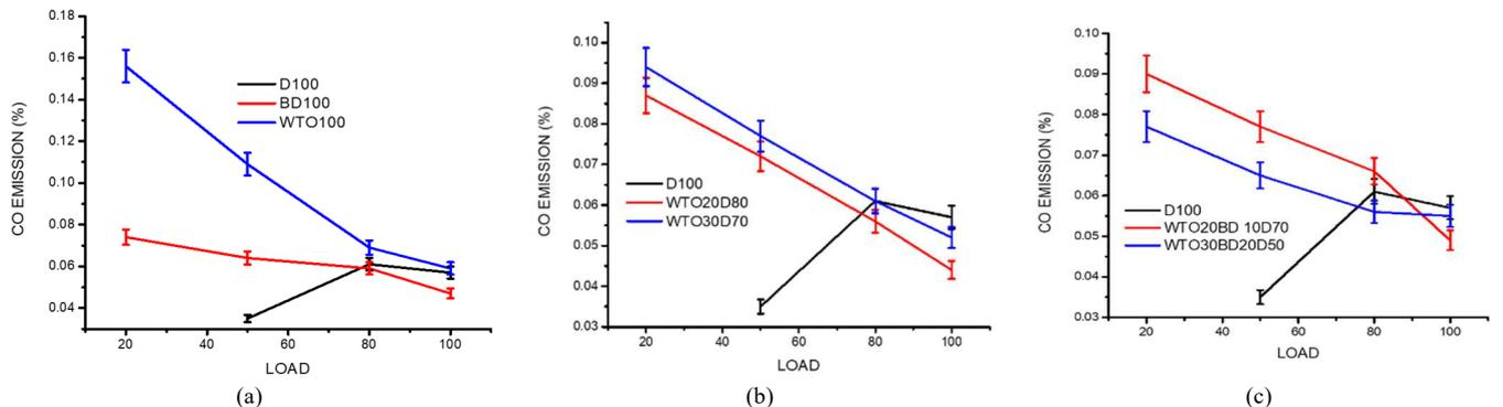
Fig. 24 (a) Carbon Monoxide emission vs. load for Base fuels; (b) Carbon Monoxide emission vs. load Base fuels and WTO with Diesel blends; (c) Carbon Monoxide emission vs. load WTO with biodiesel and Diesel blends
