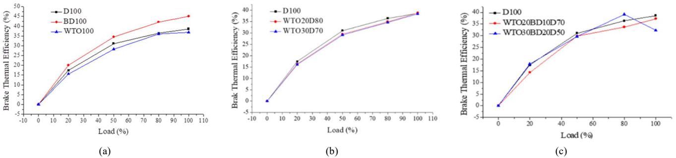
Fig. 17 (a) BTE vs. load for Base fuels, (b) BTE vs. load Base fuels and WTO with Diesel blends, (c) BTE vs. load WTO with biodiesel and Diesel blends
