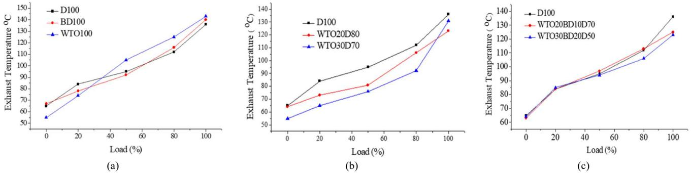
Fig. 22 (a) Exhaust temperature vs. load for Base fuels; (b) Exhaust temperature vs. load Base fuels and WTO with Diesel blends; (c) Exhaust temperature vs. load WTO with biodiesel and Diesel blends
