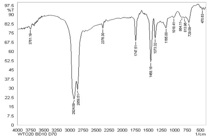
Fig. 15 FTIR analysis of WT020BD10D70
