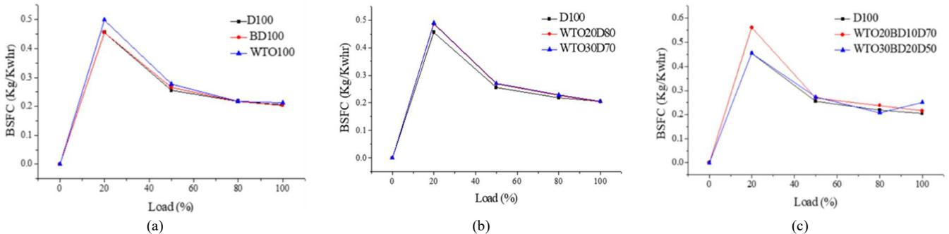
Fig. 18 (a) BSFC vs. load for Base fuels; (b) BSFC vs. load Base fuels and WTO with Diesel blends; (c) BSFC vs. load WTO with biodiesel and Diesel blends
