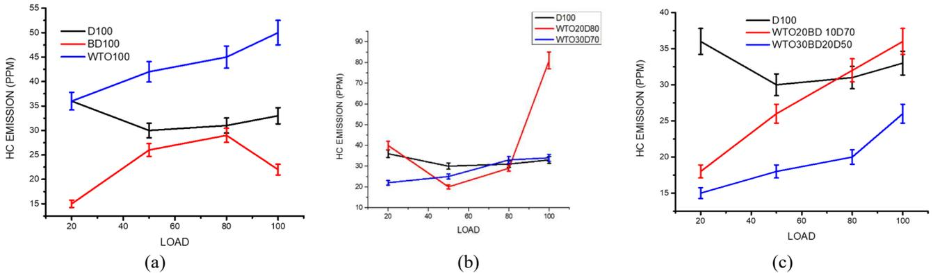
Fig. 23 (a) Hydrocarbon emission vs. load for Base fuels; (b) Hydrocarbon emission vs. load Base fuels and WTO with diesel blends; (c) Hydrocarbon emission vs. load WTO with biodiesel and Diesel blends
