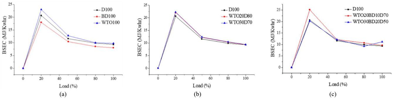
Fig. 19 (a) BSEC vs. load for Base fuels; (b) BSEC vs. load Base fuels and WTO with Diesel blends; (c) BSEC vs. load WTO with biodiesel and Diesel blends
