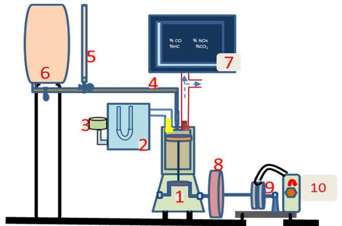
Fig. 3 Schematic diagram of the test engine (1 - Engine, 2 - Air-box with manometer, 3 - Air filter, 4 - Fuel Line, 5 - Fuel burette, 6 - Fuel Tank, 7 - Exhaust Gas Analyzer, 8 - Flywheel, 9 - Eddy-current dynamometer, 10 - Dynamometer Control)
