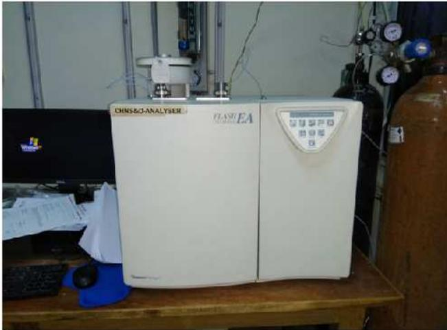
Fig. 1 CHN - Elemental analyzer
