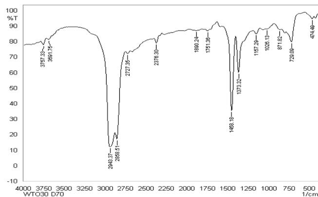
Fig. 14 FTIR analysis of WTO30D70
