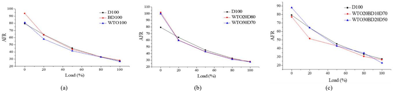
Fig. 21 (a) Air fuel ratio vs. load for Base fuels; (b) Air fuel ratio vs. load Base fuels and WTO with Diesel blends; (c) Air fuel ratio vs. load WTO with biodiesel and Diesel blends
