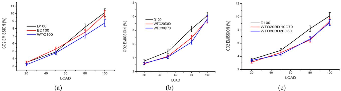
Fig. 26 (a) Carbon Dioxide emission vs. load for Base fuels; (b) Carbon Dioxide emission vs. load Base fuels and WTO with Diesel blends; (c) Carbon Dioxide emission vs. load WTO with biodiesel and Diesel blends
