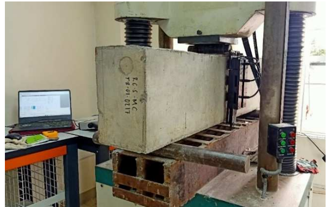
Fig. 4 Ultrasonic transducer attached to the RC beam
