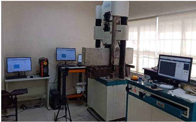
Fig. 5 Flexural strength test of RC beam while simultaneously measuring the ultrasonic pulses
