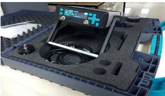
Fig. 3 PUNDIT Lab + with 54 kHz Ultrasonic Transducers
