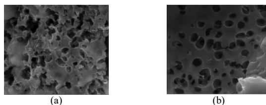
Fig. 2 a) KOH 1 M with T=600°C, b) KOH 1 M with T=700°C
