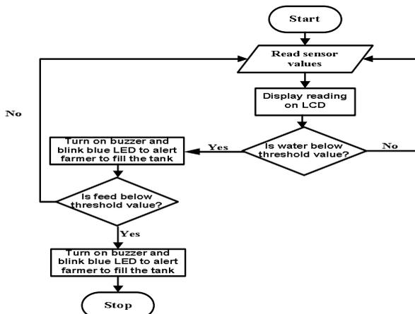
Fig. 7 Flowchart for water and feed level control unit
