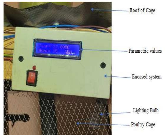
Fig. 15 Ambient temperature and humidity values on the LCD screen outside the poultry chamber
