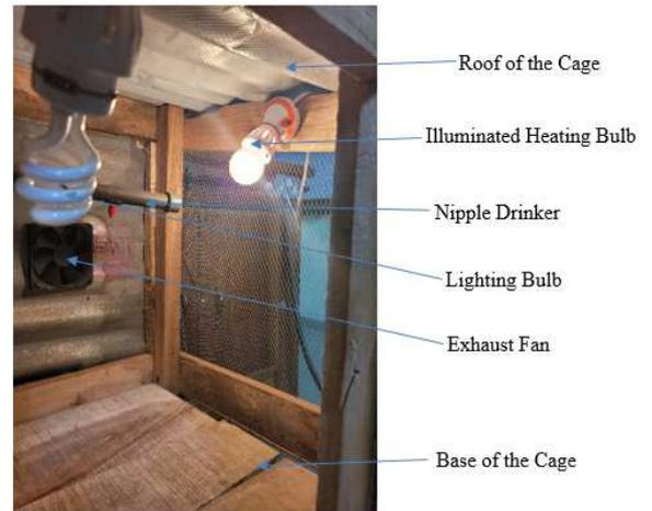
Fig. 14 Illuminated heating bulb in the poultry chamber
