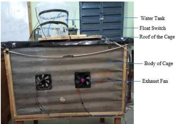
Fig. 11 Rear view of the developed poultry regulating system
