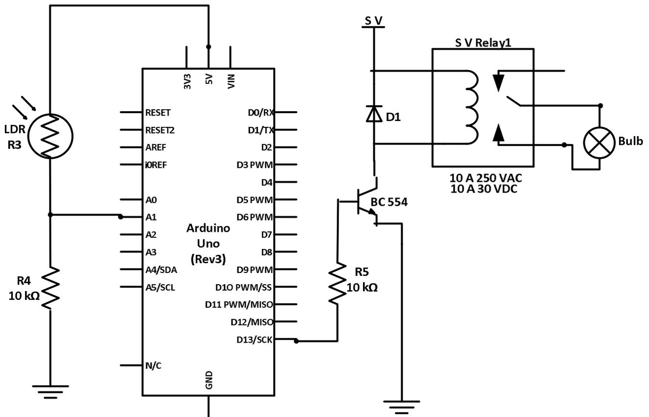
Fig. 3 Circuit diagram of the smart lighting unit
