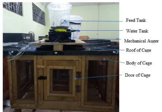
Fig. 9 Front view of the developed poultry regulating system
