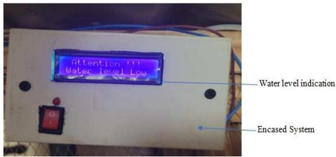
Fig. 16 Water level indication displayed on the LCD screen outside the poultry chamber
