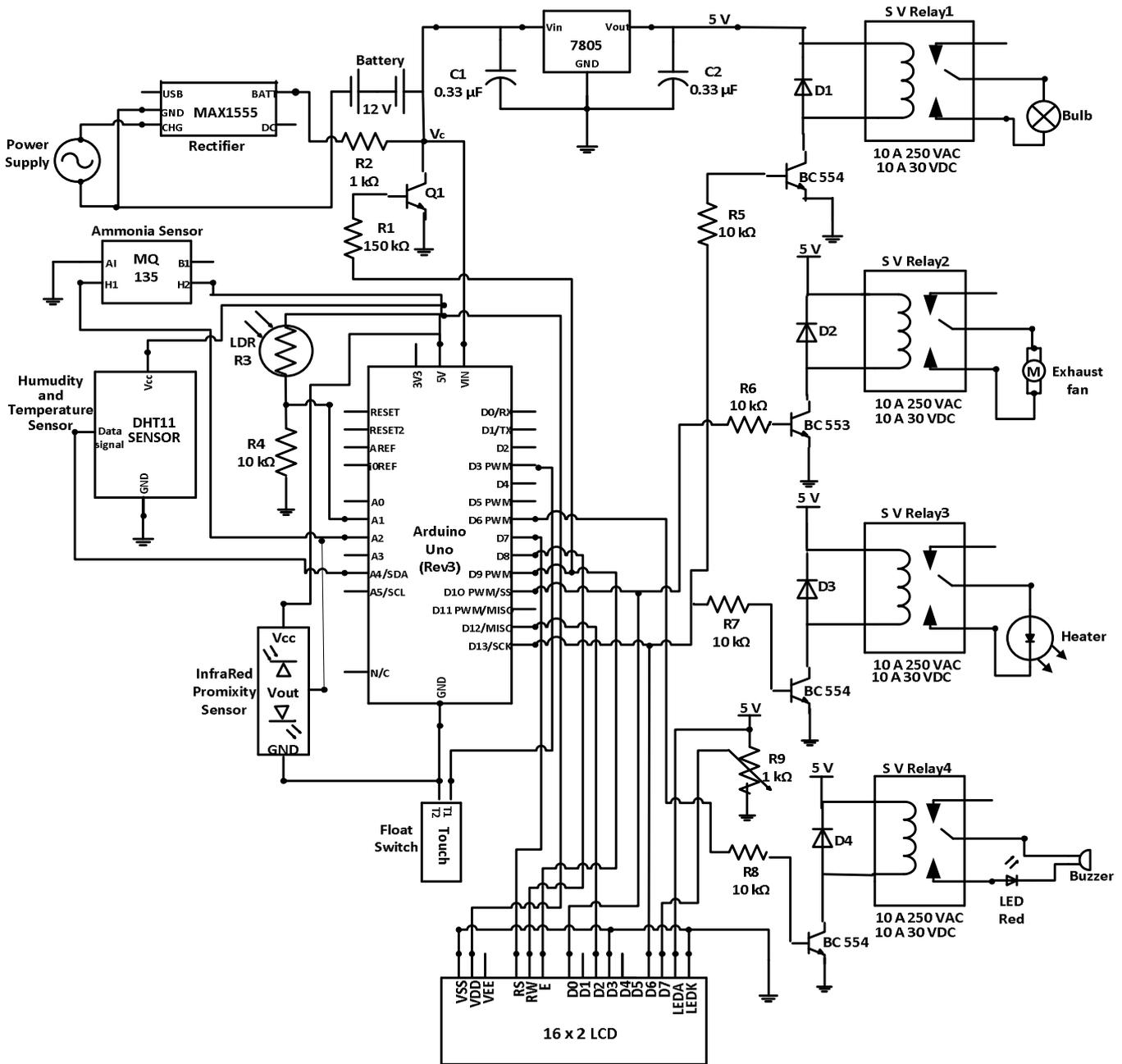
Fig. 8 Circuit diagram of the automated poultry regulating system
