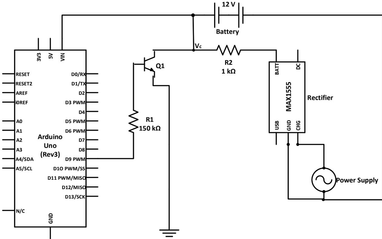
Fig. 2 Circuit diagram of the power supply unit
