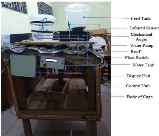
Fig. 10 Side view of the developed poultry regulating system
