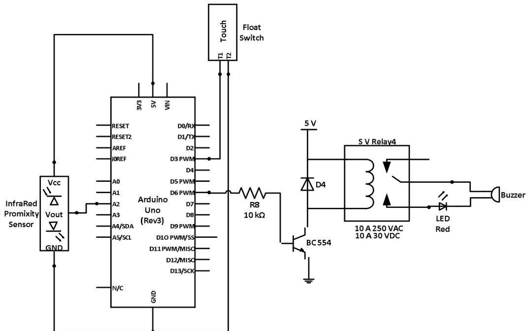
Fig. 6 Circuit diagram of the water and feed level control unit
