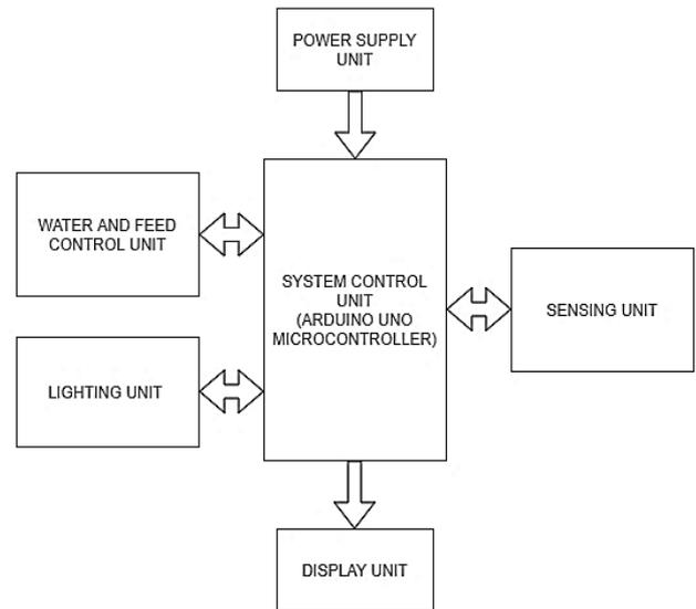
Fig. 1 Block diagram of an automated poultry regulating system
