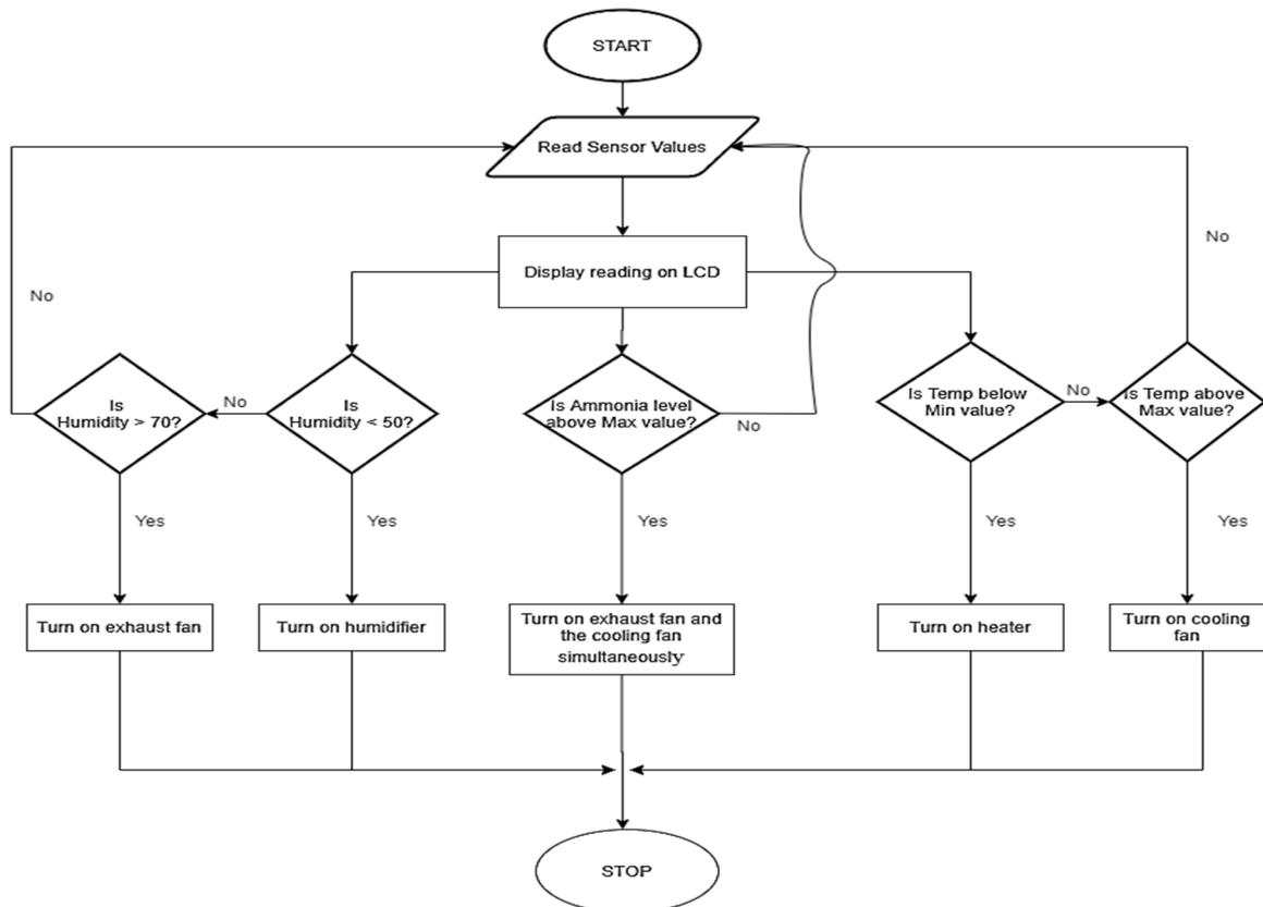
Fig. 5 Flowchart for sensing unit
