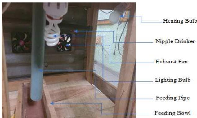
Fig. 12 Interior of the cage with output devices
