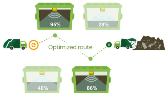
Fig. 6 Enevo's sensor can route collection to where it most needs it.
