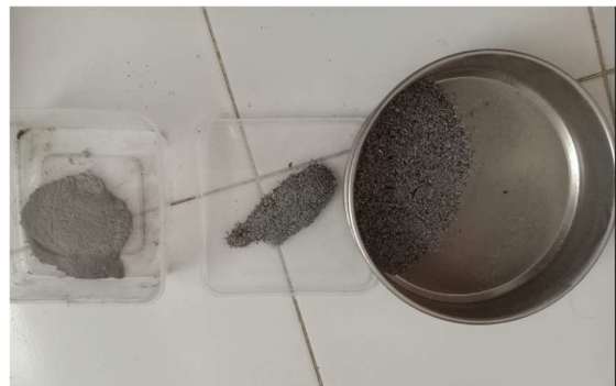
Fig. 11 Rice husk ash filtration
