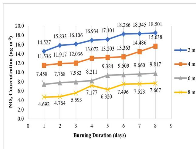
Fig. 16 Relation between burning duration and NO<sub>2</sub> concentration at various measurement distances (sampling point 1)
