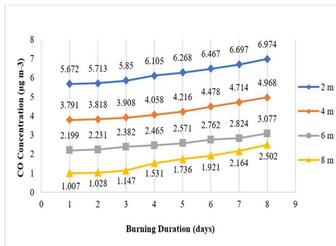
Fig. 14 Relation between burning duration and CO concentration at various measurement distances (sampling point 2)
