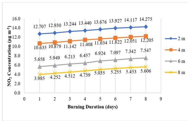
Fig. 17 Relation between burning duration and NO<sub>2</sub> concentration at various measurement distances (sampling point 2)
