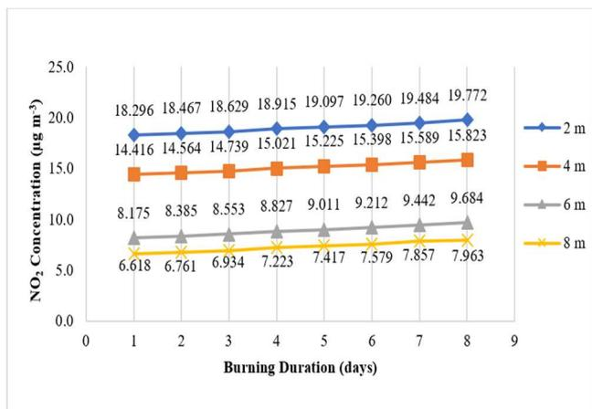
Fig. 18 Relation between burning duration and NO<sub>2</sub> concentration at various measurement distances (sampling point 3)
