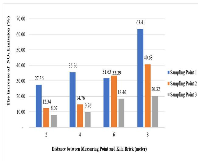
Fig. 20 The increase in NO<sub>2</sub> concentration at the three sampling points
