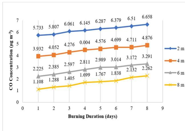
Fig. 13 Relation between burning duration and CO concentration at various measurement distances (sampling point 1)
