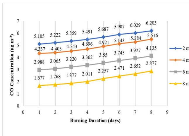
Fig. 15 Relation between burning duration and CO concentration at various measurement distances (sampling point 3)
