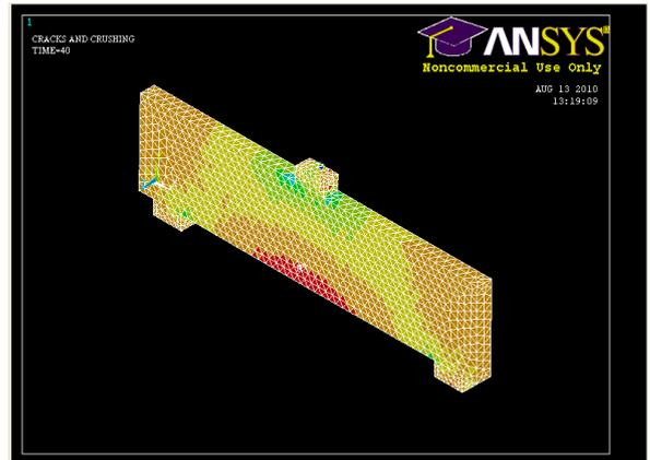
Fig. 4 Increase cracking at the wall panel
