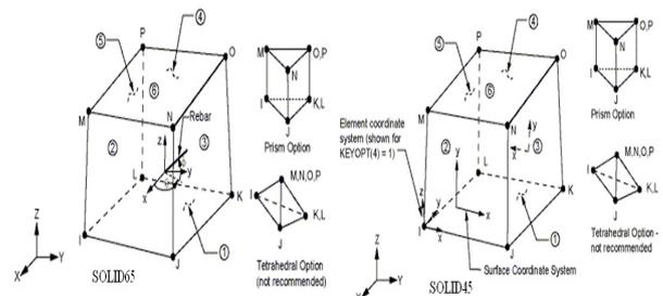
Fig. 1 SOLID65 and SOLID45 geometry
