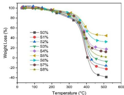
Fig. 5 Thermal Gravimetric Analysis curve of the test sample
