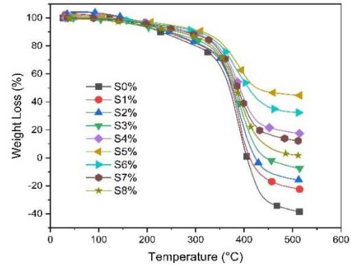
Fig. 5 Thermal Gravimetric Analysis curve of the test sample
