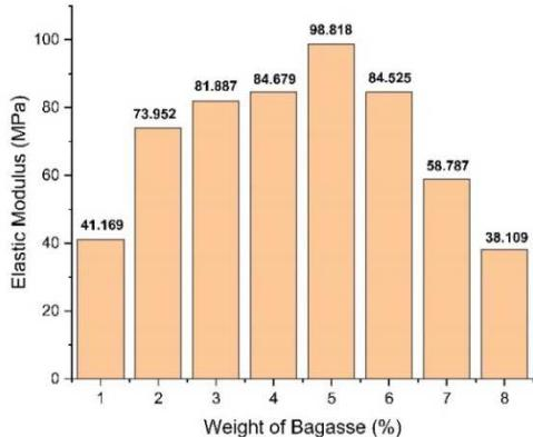
Fig. 4 Modulus of elasticity of the bagasse fiber
