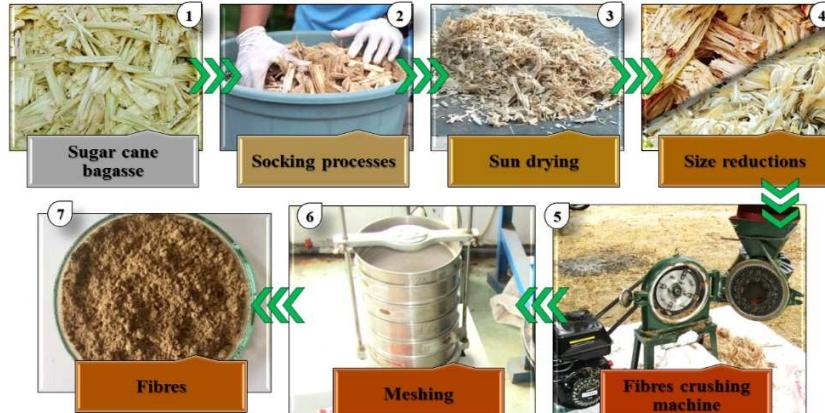
Fig. 1 Stages of the process of making bagasse fibers
