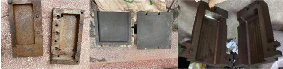
Fig. 1 Metal molds are designed for large and small batches [50]
