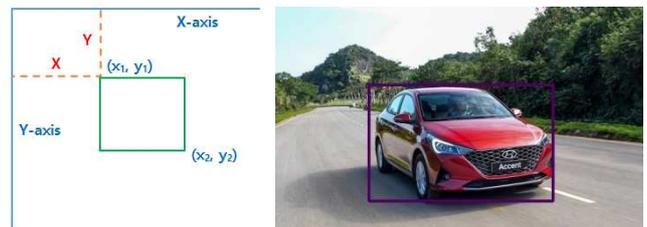
Fig. 8 ROI in object detection
