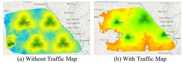
Fig. 9 Comparison RSRP frequency 700 MHz+26 GHz
