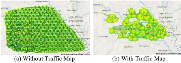
Fig. 11 Comparison SINR frequency 26 GHz
