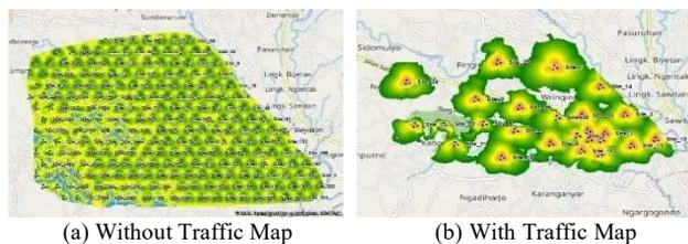
Fig. 8 Comparison RSRP frequency 26 GHz
