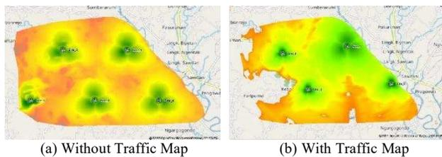
Fig. 7 Comparison RSRP frequency 700 MHz
