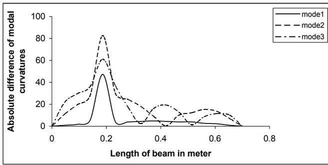
Fig.6 ADMC between cracked and un-cracked beam having crack of 5 cm depth at 0.25L
