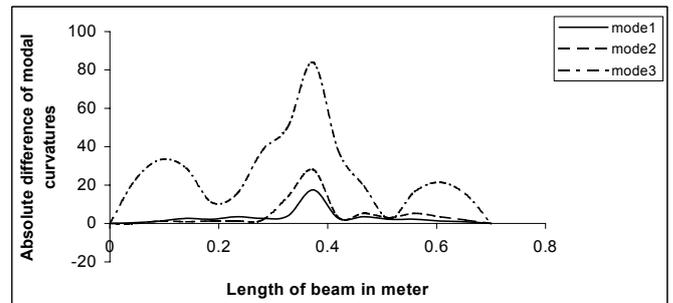
Fig.3 ADMC between cracked and un-cracked beam having crack of  $3 \text{ cm}$  depth at  $0.5L$
