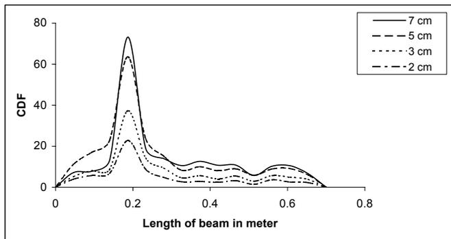
Fig.14 CDF for beam having different crack depths at 0.25L
