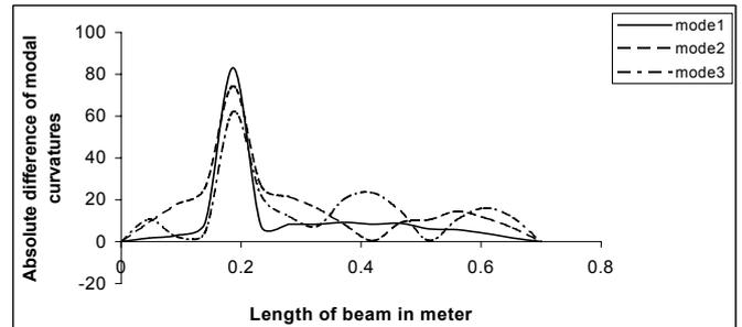
Fig.5 ADMC between cracked and un-cracked beam having crack of  $7 \text{ cm}$  depth at  $0.25L$
