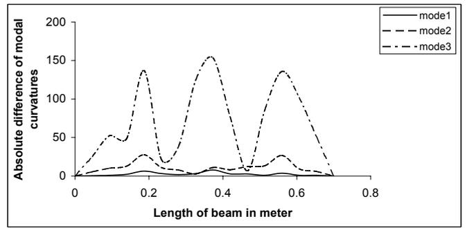
Fig.11 ADMC between cracked and un-cracked beam having multiple cracks of 3 cm depth at 0.25L, 0.5L and 0.75L
