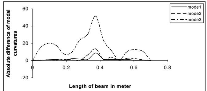
Fig.4 ADMC between cracked and un-cracked beam having crack of  $2 \text{ cm}$  depth at  $0.5L$
