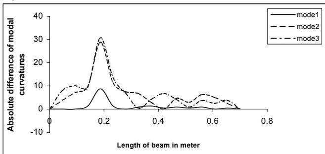
Fig.8 ADMC between cracked and un-cracked beam having crack of 2 cm depth at 0.25L
