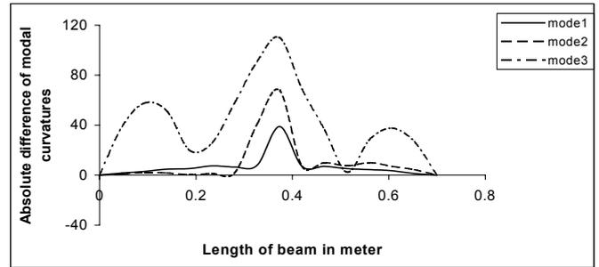
Fig.2 ADMC between cracked and un-cracked beam having crack of  $5 \text{ cm}$  depth at  $0.5L$
