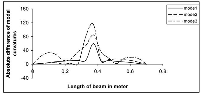
Fig.1 ADMC between cracked and un-cracked beam having crack of  $7 \text{ cm}$  depth at  $0.5L$
