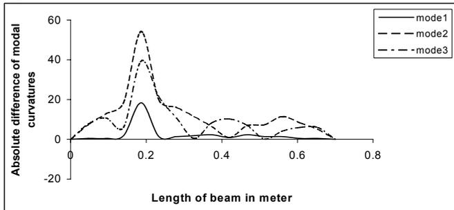
Fig.7 ADMC between cracked and un-cracked beam having crack of 3 cm depth at 0.25L
