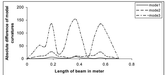
Fig.12 ADMC between cracked and un-cracked beam having multiple cracks of 2 cm depth at 0.25L, 0.5L and 0.75L
