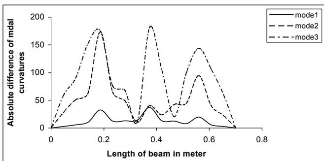
Fig.9 ADMC between cracked and un-cracked beam having multiple cracks of 7 cm depth at 0.25L, 0.5L and 0.75L
