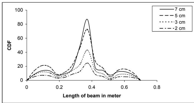
Fig.13 CDF for beam having different crack depths at 0.5L
