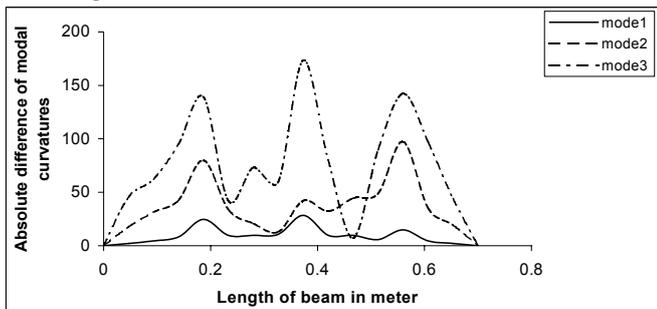
Fig.10 ADMC between cracked and un-cracked beam having multiple cracks of 5 cm depth at 0.25L, 0.5L and 0.75L
