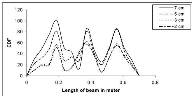
Fig.15 CDF for beam having different crack depths at 0.25L, 0.5L and 0.75L
