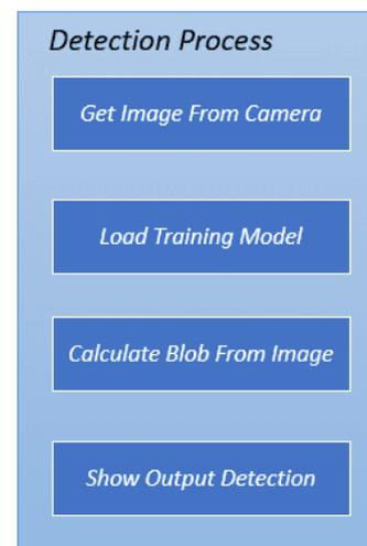
Fig. 6 Landmark Detection Process
